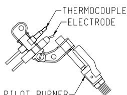
to light pilot). Continue to hold the control knob in for about one (1) minute after the pilot is lit. Release knob and it will pop back up. Pilot should remain lit. If it goes out, repeat steps 3 through 7.
