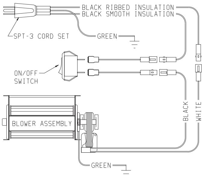
If any of the original wire as supplied with the appliance must be replaced, it must be replaced with type 125°C wire or its equivalent.
